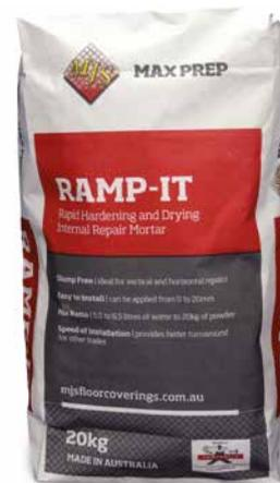
MJS Ramp-It is workable for approx. 20 minutes at 18 – 20°C. Lower temperatures lengthen the working time, higher temperatures shorten it. MJS Ramp-It is particularly suited for restoring worn out and damaged steps and stairs. After approx. 20 minutes trim off excess mortar and finish off with a wet trowel, sponge or float to obtain a smooth surface.
