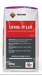
**Application** | Cementitious underlayment for repairing internal cement floors **Easy to install** | 2.5mm to 10mm in one application **Mixing ratio** | 4.5 litres of water to 20kg powder **Coverage** | 20kg bag covers 4m<sup>2</sup> at 3mm thickness
