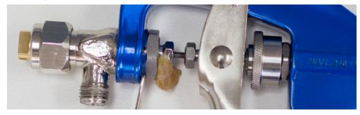
The adhesive only passes through a very small part of the gun when being sprayed. To prevent the adhesive from leaking out of this area, it is sealed off. This seal is held in place by a nut. Over time, this can become loose, causing the seal to fall out of place. This needs to be tightened. However, be careful not to make this to tight, as it will mean the trigger will not work, and the adhesive won't spray as it should.
