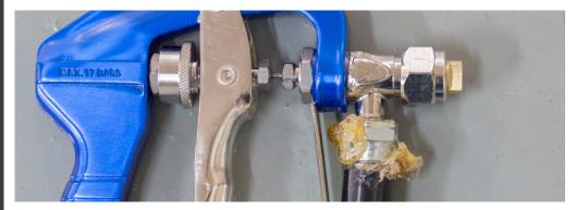
If so, it is too loose and needs tightening. The gun and hose are designed to join almost seamlessly together. This is to provide the adhesive with a straight, unbroken trajectory to the gun tip. Any breaks in this line will mean the adhesive will leak out.
