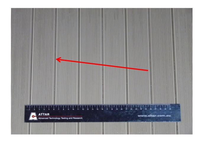
Figure 1: ASNPI Aluminum Tread Plate stair nosing Arrow indicates direction of testing
