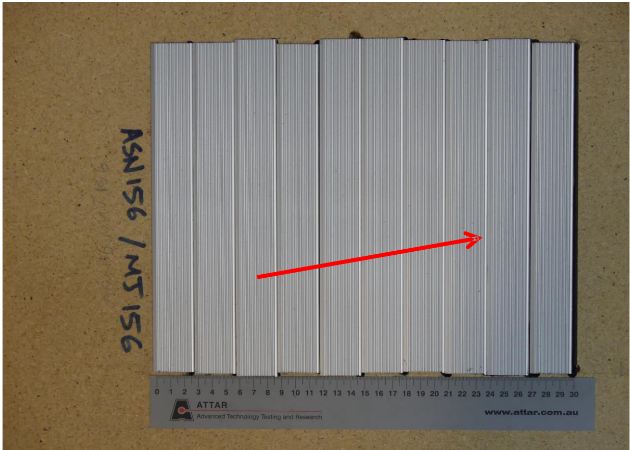
Figure 1: ASN156 / MJ156 stair nosing Arrow indicates direction of testing
