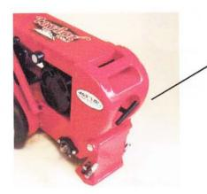
Loosen and remove "T" Bolt to remove front weight.
