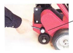
Rachet fastener secures base weight. Pull knob out to rachet handle position.
