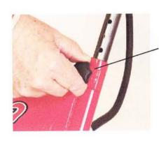
Release handle bar by pulling up on both knobs simotaneously. Then extend or collapse handle bar.
