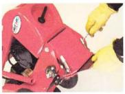
Wear cut resistant gloves when installing or removing blade.
