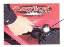
Rachet fastener secures hood weight. Pull knob out to rachet handle position.
