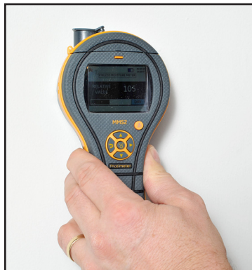
Figure 3: Taking Relative Moisture Readings
