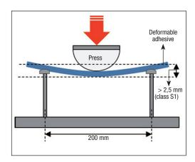
By mixing **Rapid S1 Tile Adhesive** with **Latex Plus** the deformability improves, to meet the requirements of class C2F S2 (highly deformable, fast setting, improved cementitious adhesive) according to AS ISO 13007.1.
